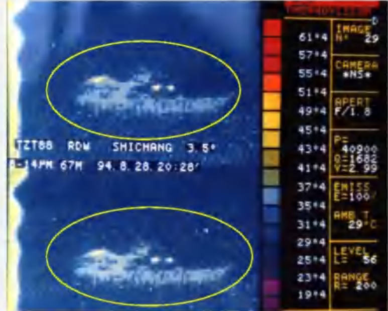
Infrared image : Tank is camouflaged by anti-infrared camouflage net
